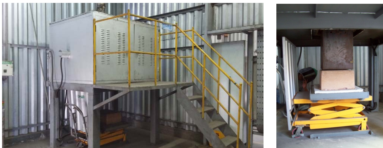
Figure 2. Left: General aspect of the pilot coke oven. Right: Charging of the coal cake in a box through the bottom of the oven, using a hydraulic lifting car.
