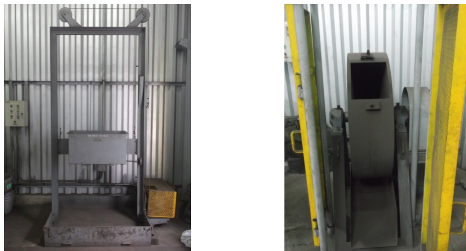
Figure 5. Equipment for shatter test (left) and ¼ MICUM test (right).
