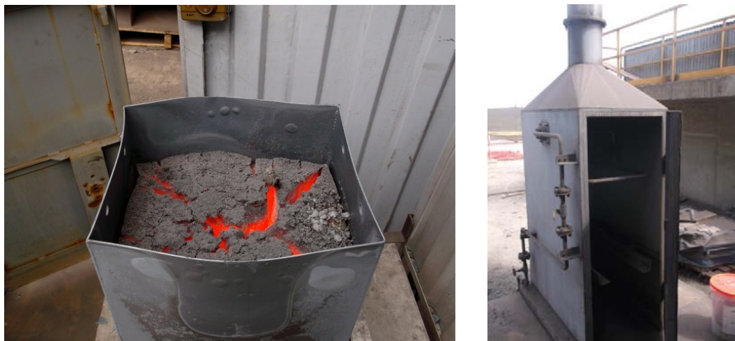
Figure 4. Steel box with incandescent coke after discharge from the oven. Right: quenching tower.
